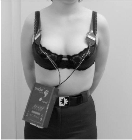
7.7 Novel pliance-sensor pressure strips. Source: Novel's Pliance [8].
