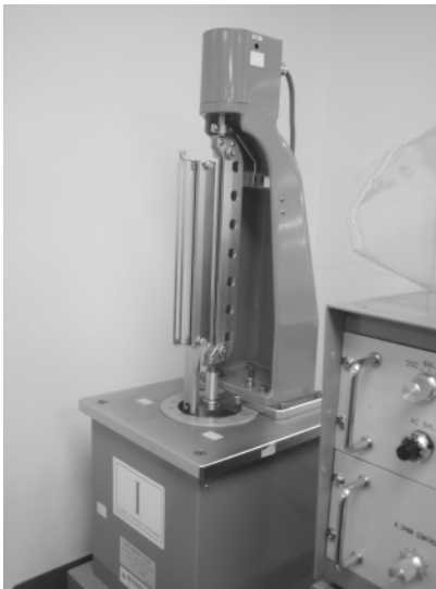
9.9 KES-F2 bending tester.
