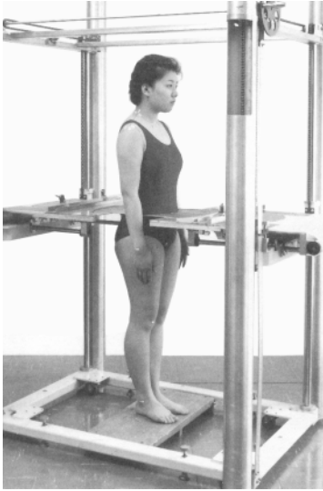
2.4 The horizontal sliding gauge. Source: Miyoshi M, Clothing construction, Bunka Publishing Bureau, 2001 [7].
