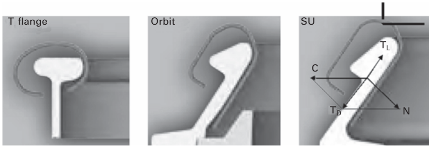
7.4 Types of ring and traveller (courtesy of Bracker).
