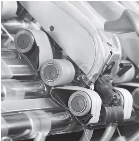
9.13 Self-cleaning apron in Zinser CompACT 3 ® system.
