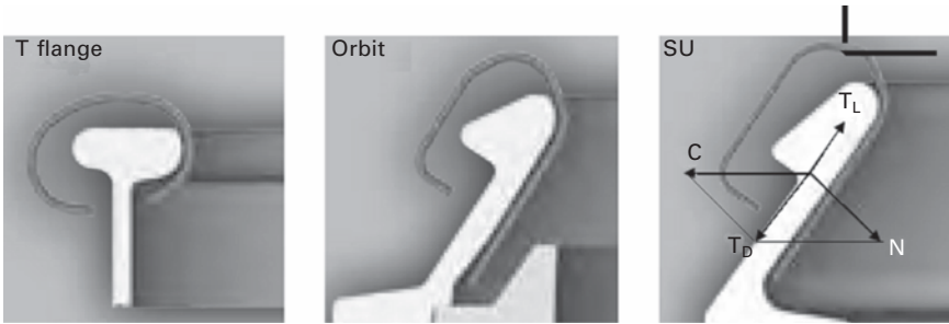
2.9 Ring and traveller combinations (courtesy of Bracker).
