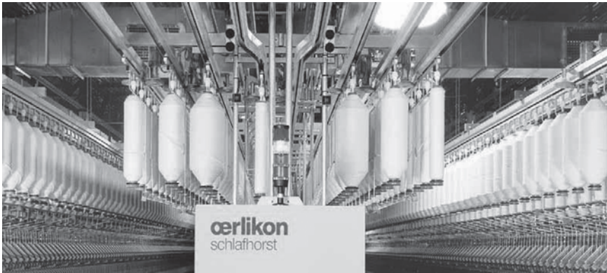
7.11 Automatic transfer of roving bobbin with rows of creel: CimTrack 4 (courtesy of Oerlikon Schlafhorst Zinser).
