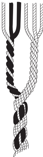
6.9 Direction of twist and construction of plied and cord (cabled) yarn (source: Methods of Test for Textiles , British Standards Institution, Handbook No. 11, 1963, British Standards House, London).
