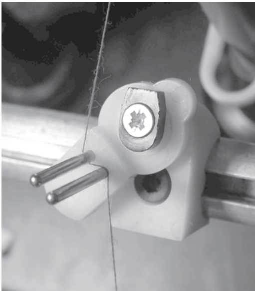
8.3 Sirospun break-out device.
