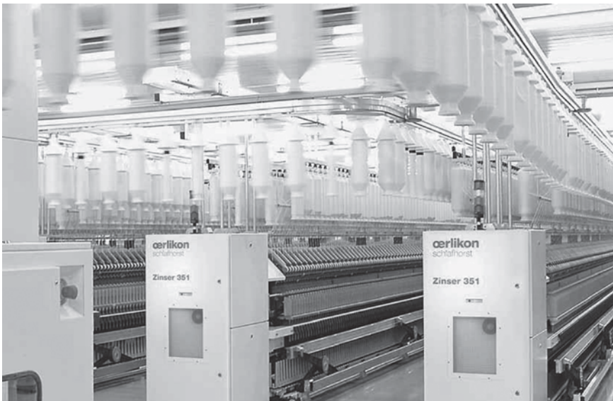
7.12 Ring spinning machine with automatic roving bobbin transfer (courtesy of Oerlikon Schlafhorst Zinser).
