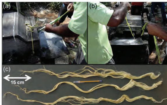
FIGURE 2.4 Extraction of PALF by mechanical process using a decorticator machine. (a) Pineapple leaves are loaded into the decortivating machine, (b) the fibres obtained are being pulled out from the decorticator and (c) sun-dried PALFs. (Source: Reused with permission from Sena Neto et al. (2013). Copyright 2014, Elsevier, B.V.)
