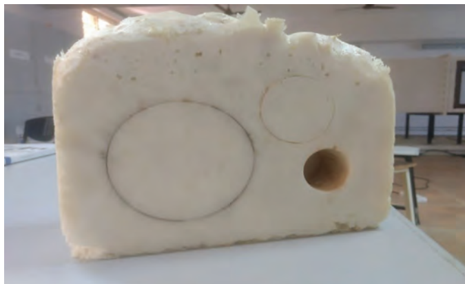
FIGURE 16.9 Open-cell PU foam incorporated with luffa fibre.
