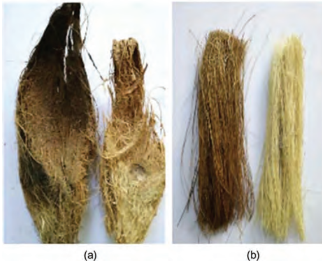
FIGURE 7.1 Brown coir (a) and white coir (b), as received and prepared for experimentation. (Source: Valášek et al. 2018.)
