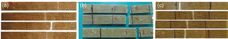
FIGURE 3.4 Tensile fracture of (a) two-layer, (b) four-layer, and (c) six-layer jute–polyester composite [62].
