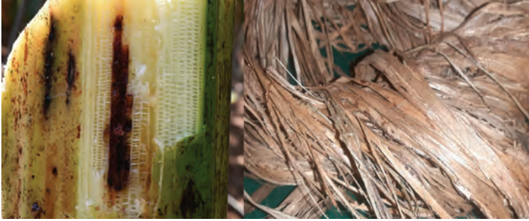
FIGURE 5.1 Tuxing technique to separate fibre from pith.
