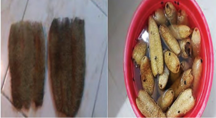
FIGURE 16.5 Pretreatment of luffa fibre with 5% of NaOH.
