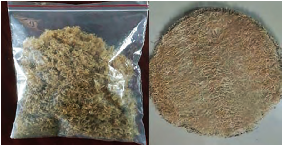
FIGURE 16.8 Short form of luffa fibre and circular shape of luffa.
