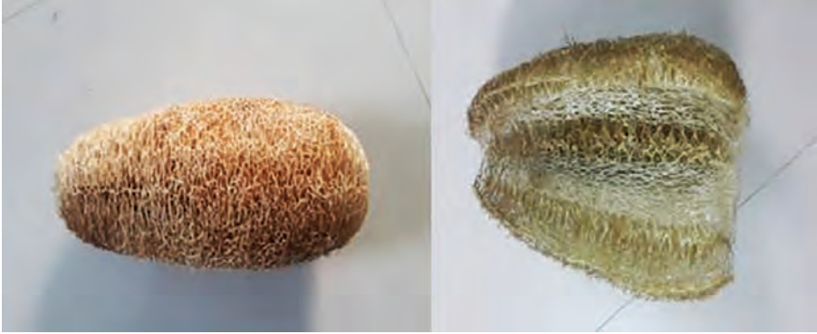
FIGURE 16.7 Separation of inner core from luffa fibre.
