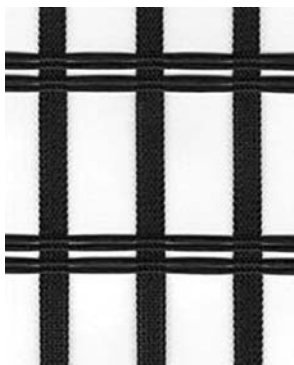
18.11 Knitted high tenacity polyester geogrids with UV stabilized saturation coating [31].
