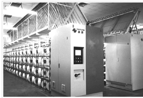
Fig. 2.19: V-type draw texturing machine
