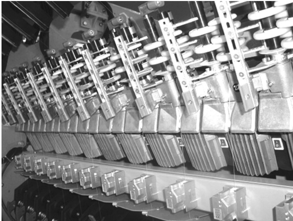
Fig. 2.22: Motorised friction units on a HY2-V texturising machine, below on-line tension measurement devices
