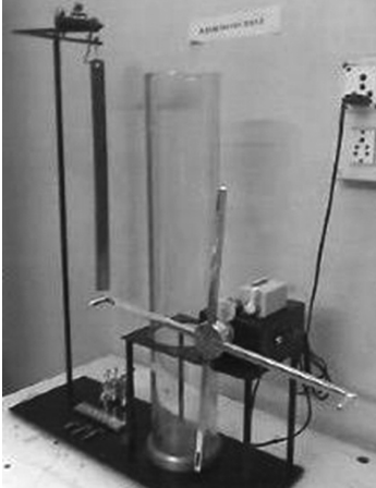
Fig. 6.3: Crimp Rigidity Tester by B. Tex Testing
