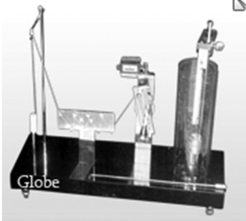
Fig. 6.4: Crimp rigidity tester by Globe enterprises
