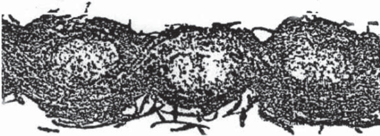
3.13 Cross-section image of plain-weave fabric containing two consecutive yarns.
