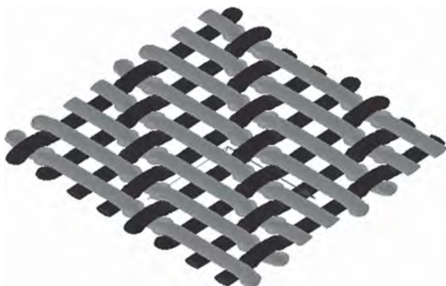
FIGURE 5.14 Interlacement pattern in a 3/1 twill weave (warp: grey and weft: black).
