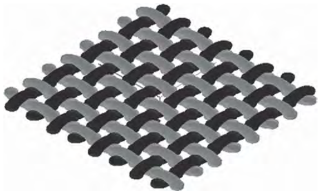
FIGURE 5.5 Interlacement pattern of a plain weave (warp: grey and weft: black).
