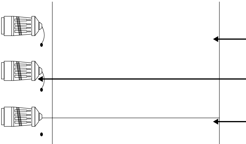
FIGURE 8.47 Steps of weft insertion by rigid rapier.
