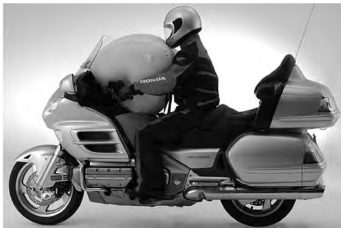
8.17 Use of nylon 6.6 fibre for an airbag as a passive safety system in a motorcycle (Source: Honda Motorcycle Business Literature, 2006).
