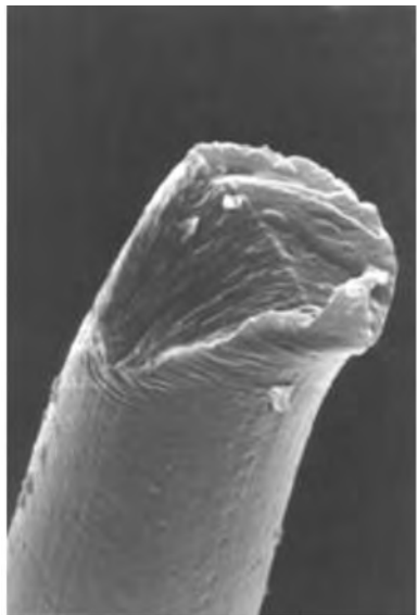
8.14 Scanning electron micrograph of one side of a highly drawn nylon 6.6 filament broken in tension (courtesy: Professor A R Bunsell).
