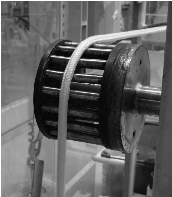
13.15 Cover surface abrasion test using a rotating spoke wheel.
