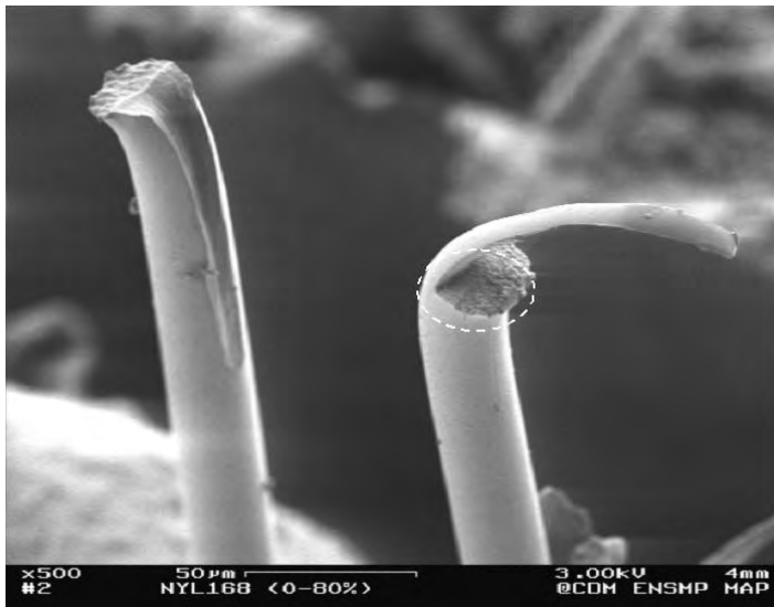
11.4 The tongue end of a PET fibre broken at room temperature at 50 Hz revealing the very long crack development before failure. The diameter of the fibre was 18 μm and the length of the crack was 2.4 mm.
