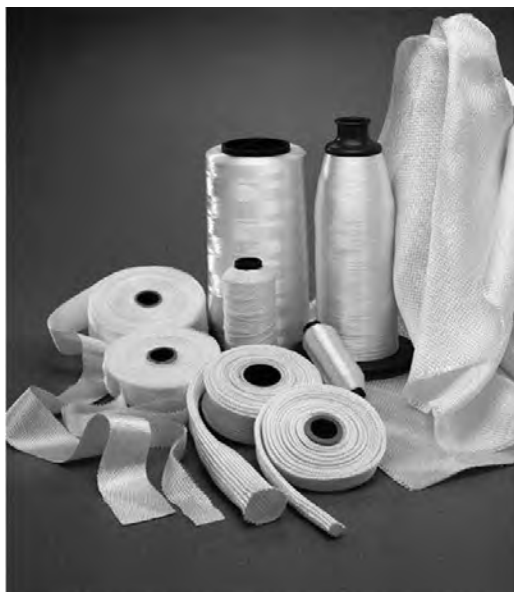
18.1 Continuous rovings, fabrics and braided sleeving of ceramic oxide fibers.
