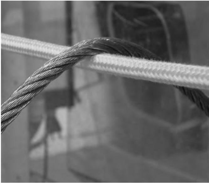
13.16 Rope cover sawing test using a steel wire.
