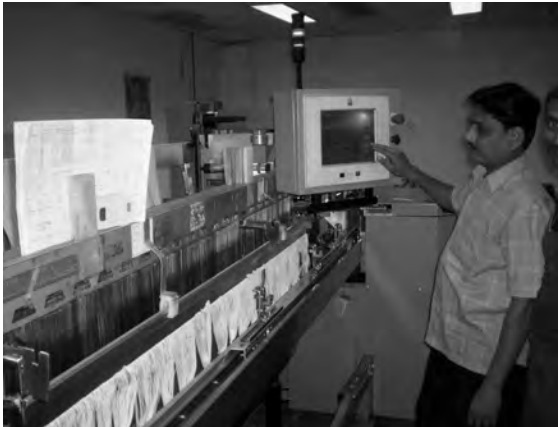
Automatic drawing-in machine.
