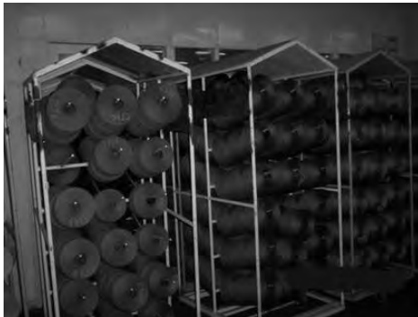
Proper storing of double yarn material to prevent spoilage of upper layers.
