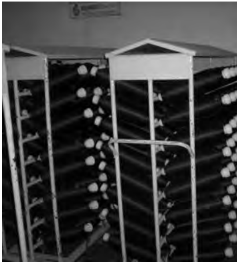
Proper storing of roving materials in trolleys to prevent spoilage of upper layers.
