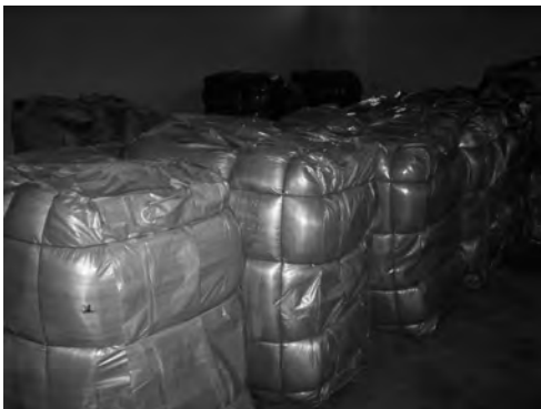
Tops sliver, kept in compressed bales, to be transported from other combing plants.
