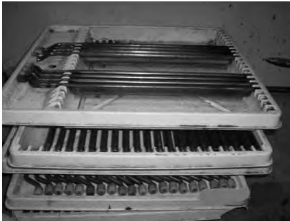
Proper keeping of soldered fallers in tray.
