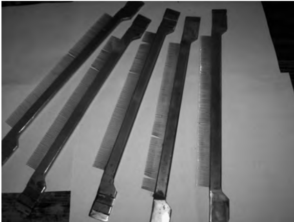
Bent, broken or missing pins in the faller.
