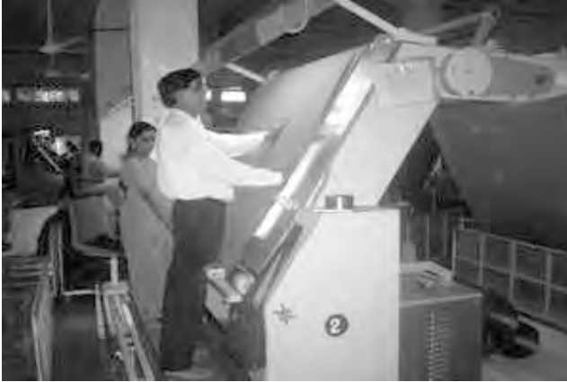
Mending table with under and over light arrangement.
