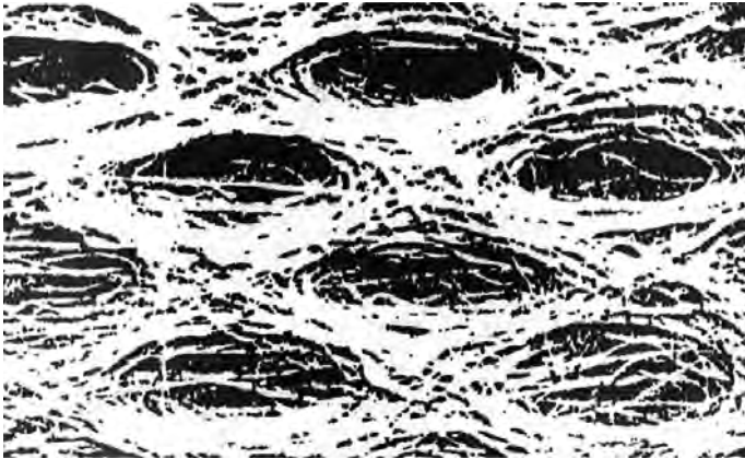
2.12 Apertured hydroentangled nonwoven structure.
