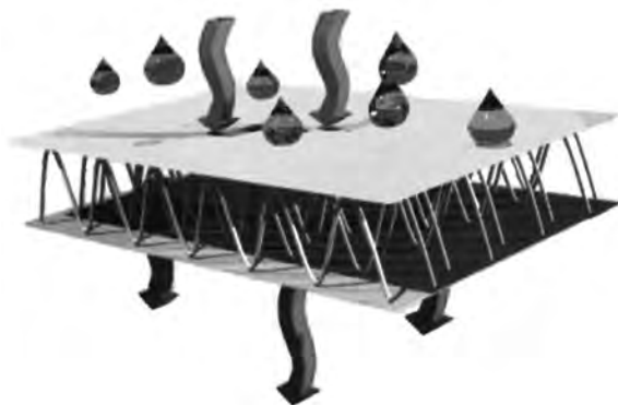
2.7 Illustration of a spacer fabric structure.
