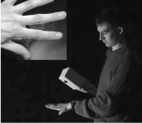
24.4 Handheld device for the electrospinning of wound dressings (Greiner and Wendorff, 2007).
