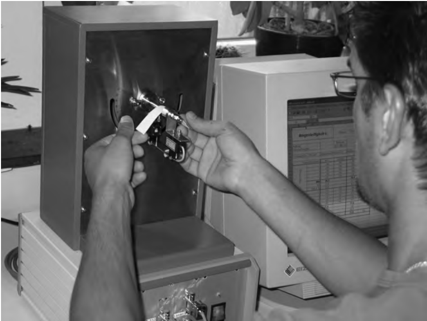
9.5 Measuring fabric's stiffness. A textile stripe is placed on a horizontal pin. Subsequently, the position of the specimen is detected by a laser beam. The bending angle of the sample is regarded as the fabric stiffness, the greater the bending angle, the stiffer the textile.
