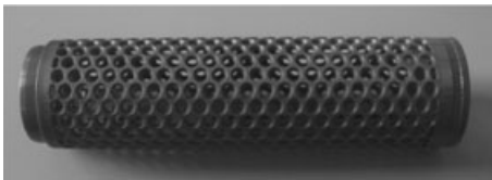
5.22 Non-compressible plastic dye tube example.
