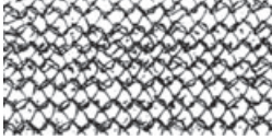
2.8 Sheer effect from torque yarn in 4-feed circular knit for ladies' hosiery. 2
