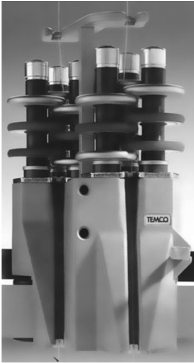
9.1 Example of twin twist unit, TEMCO FTS 4461. 1 (Photo © Oerlikon-Barmag.)
