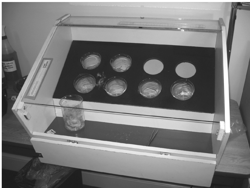
2.8 Separation cabinet (source: Peter Lieber).
