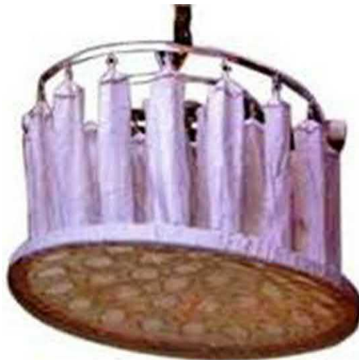
Fig. 12.6 Working position of FBD bags.
