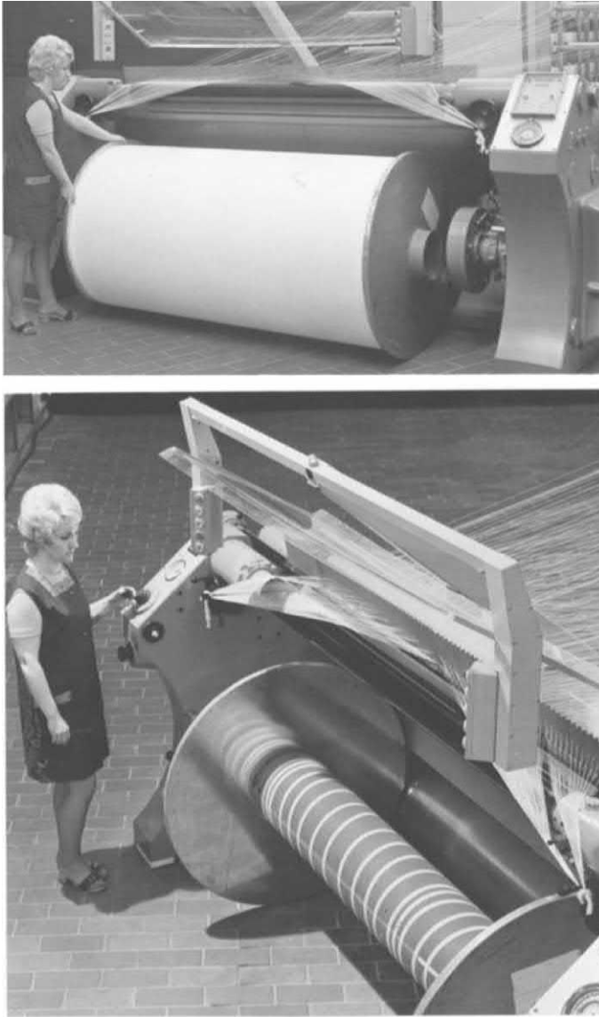
Fig. 3.3 Full beam being taken out (doffed) and new one put in.
