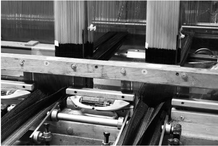
Fig. 8.69 Narrow fabric shuttle loom weaving Pi structures. Courtesy of Bally Ribbon Mills, Bally, Pennsylvania 19503, USA.
