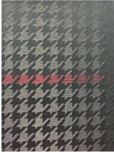
Fig. 9.8 Typical automotive jacquard seating fabric. Main features are understated design in muted self-colour and small scale to avoid dominating other interior features of the car.
