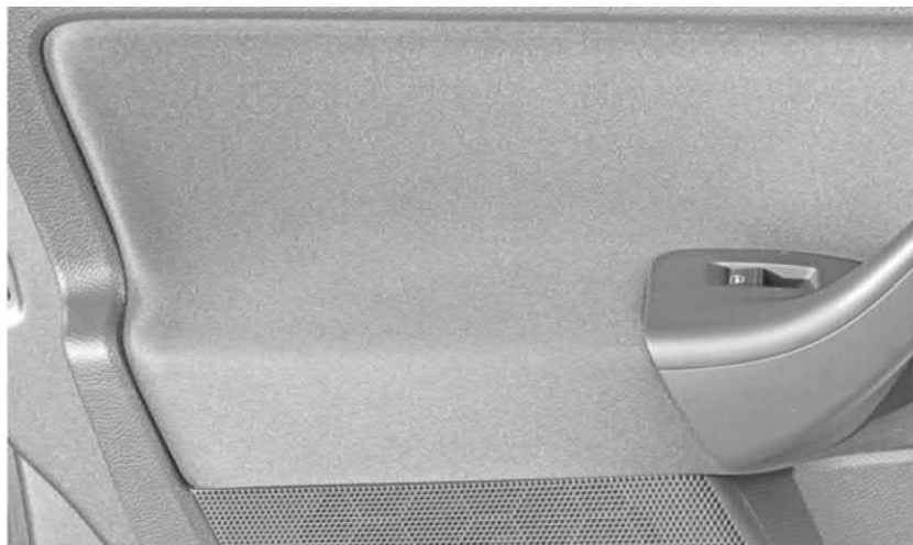
Fig. 9.5 Moulded door panel and armrest on VW Golf showing the stretch required in the fabric to mould around the deep contours. A flat woven fabric is used in the illustration.
