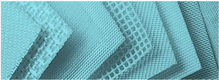
Fig. 12.2 Structures of woven filter fabrics.
