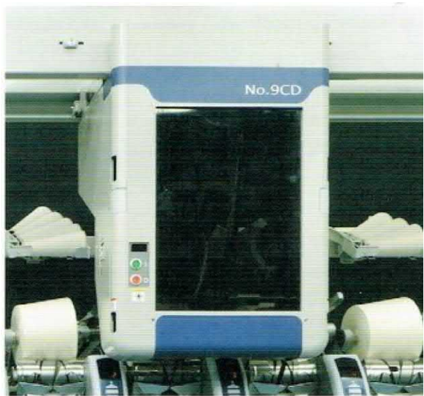
Fig. 2.26 Automatic doffer with a speed of 52 m/min.
