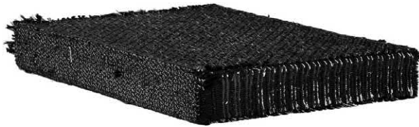
Fig. 8.9 Fifty-millimetre thick 3D orthogonal pitch panel. Courtesy of Bally Ribbon Mills, Bally, Pennsylvania 19503, USA.
