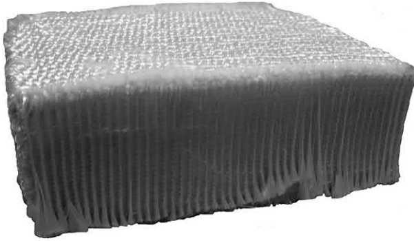
Fig. 8.8 Fifty-millimetre thick 3D orthogonal Quartz panel. Courtesy of Bally Ribbon Mills, Bally, Pennsylvania 19503, USA.
