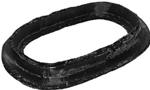
Fig. 8.26 Composite window frame.
