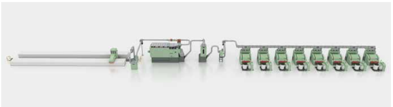
Fig. 30 – Typical blowroom line for 100 % man-made fibres
