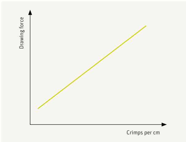
Fig. 18 – Drawing force versus intensity of crimp
