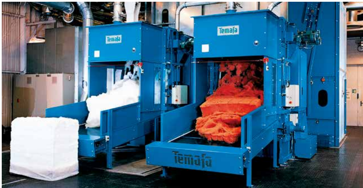
Fig. 28 – Weighing hopper feeder (Temafa)
