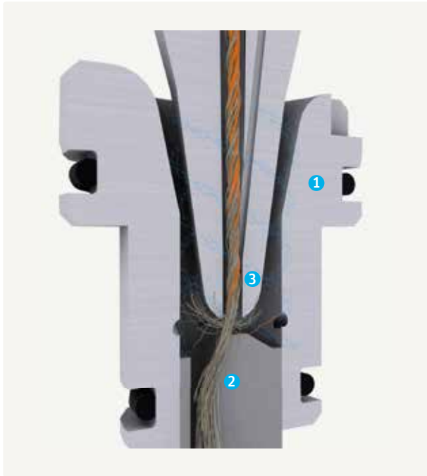
Fig. 61 – Spinning nozzle (1-housing, 2- fibre feeding element, 3-tip)
