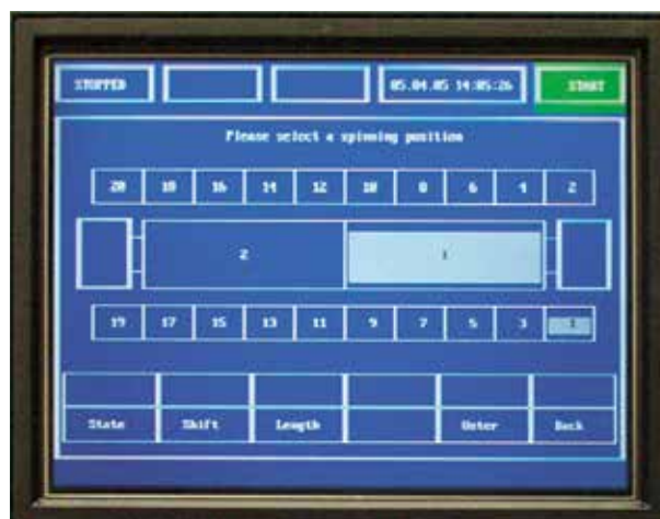
Fig. 43 – Machine operator panel in the form of a touch screen panel
