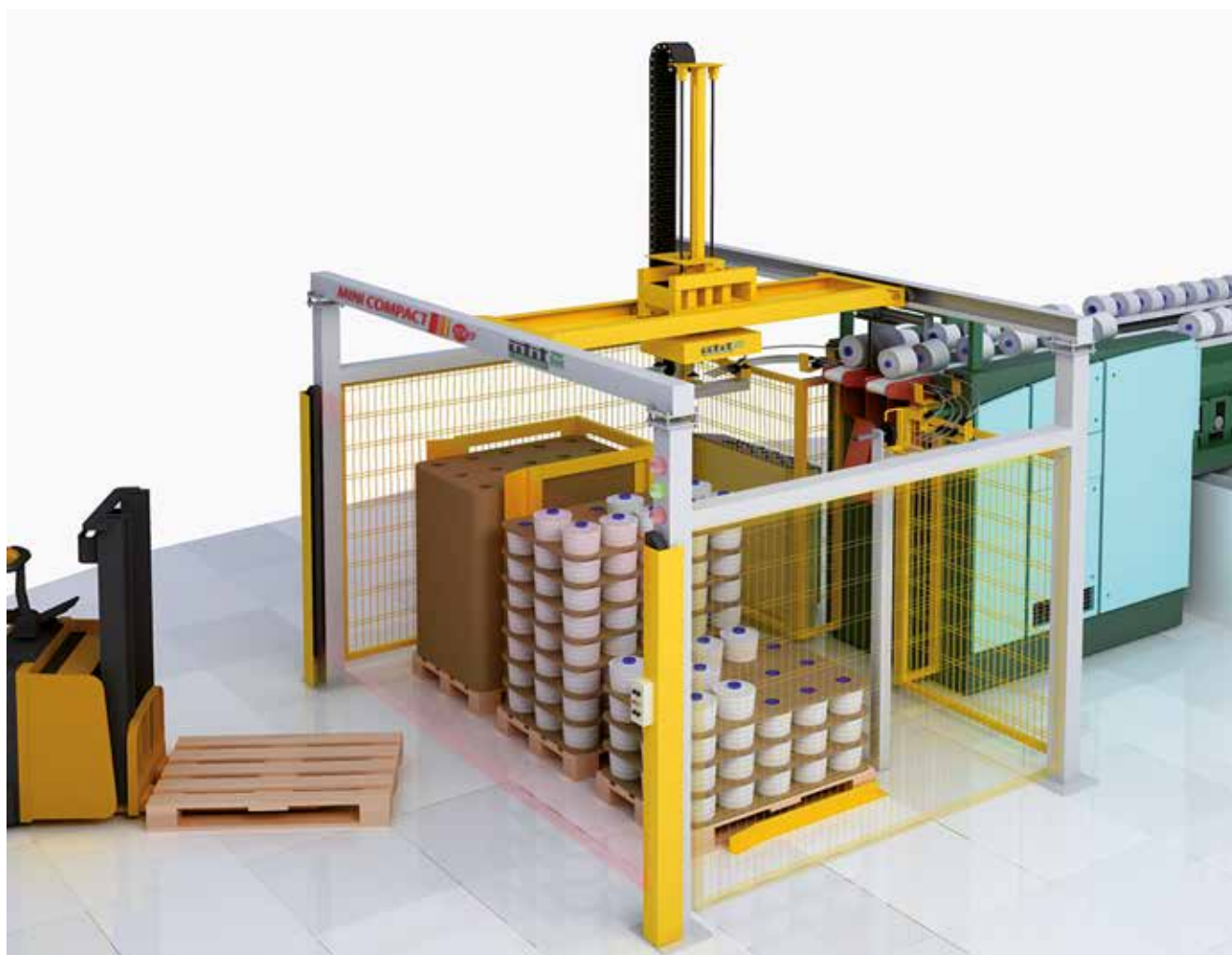
Fig. 66 – Automatic palletizing unit with protective grid on the rotor spinning machine
