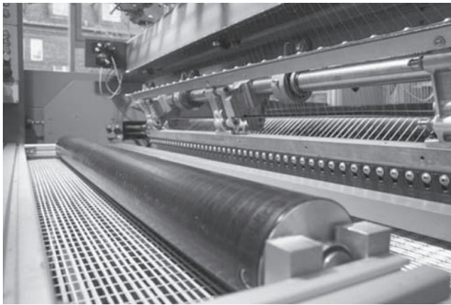
FIGURE 4.12 Coating process on the multi-axial knitting machine. (From Roye, A., Gries, T., Engler, T., Franzke, G., and Cherif, C., “Possibilities of textile manufacturing for load-adapted concrete reinforcement,” in Dubey, A. (ed.), Textile-Reinforced Concrete , Proceedings of ACI Fall Convention, Kansas City, November 2005, SP-250CD-3, CD-ROM, 2008. With permission.)
