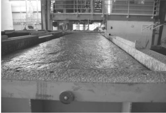
FIGURE 18.6 Fresh slurry AFRC rises inside the mold because of the hydrogen generation.
