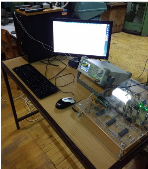
Fig. 6.14 The appearance of the developed model of the computerized scanning system for porosity deviation detection of a knitted fabric on the circular knitting textile machine
