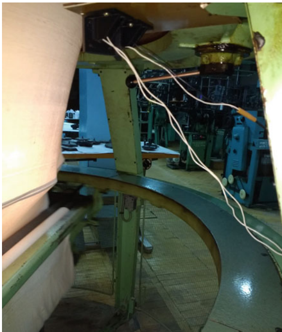
Fig. 6.15 Position of non-contact ultrasonic sensors, emitter and receiver of ultrasonic waves, relative to the knitted fabric during the operation of the circular textile machine
