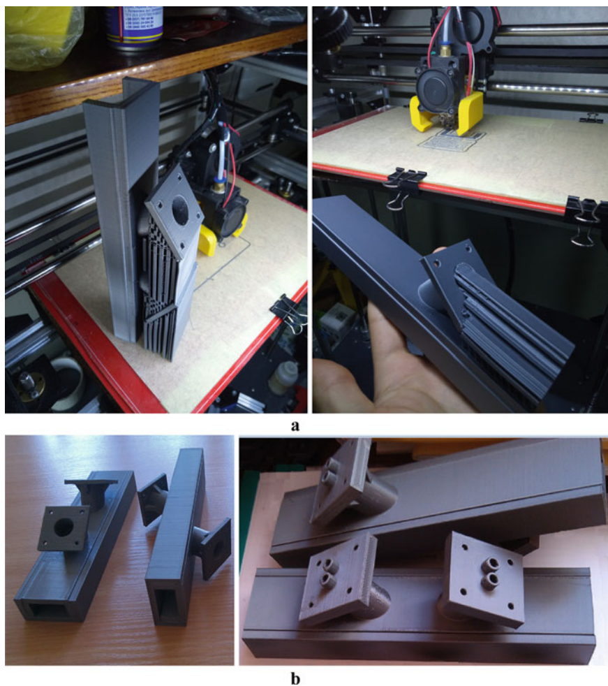
Fig. 6.6 The process of printing experimental waveguides to determine the tension of threads with high linear density on a 3D printer and the finished print result: a view of the upper parts of the waveguides after 3D printing with working support of complex shapes; b ready printed waveguides with fastenings for ultrasonic sensors both on one side of the controlled thread, and fastenings on its different sides
