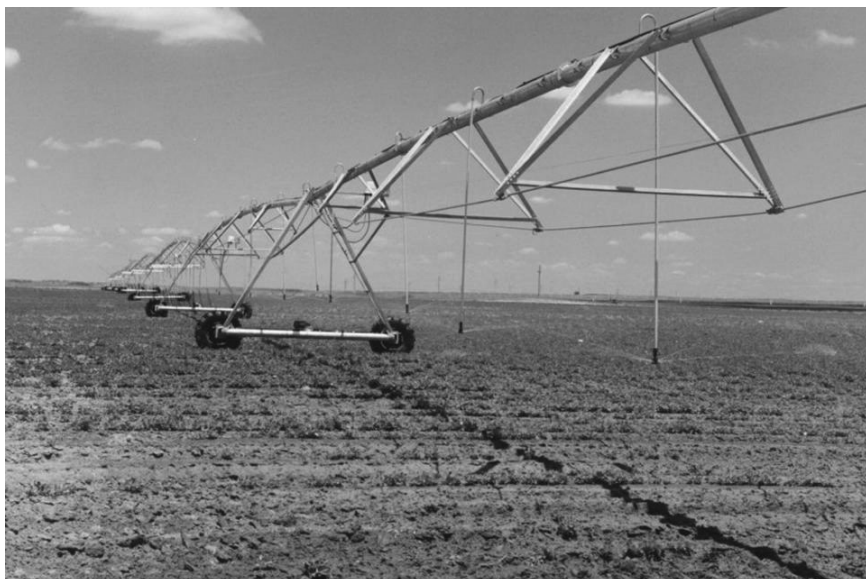
3.37 LEPA (pivot) system for irrigation of cotton plants and application of liquid agrochemicals.
