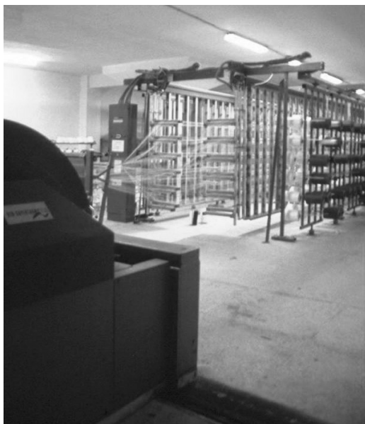
2.48 Weaving preparation: creel with yarn cones.
