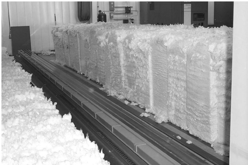
2.42 Cotton bale opening. The specific layup of the bales enables the production of a desired quality.
