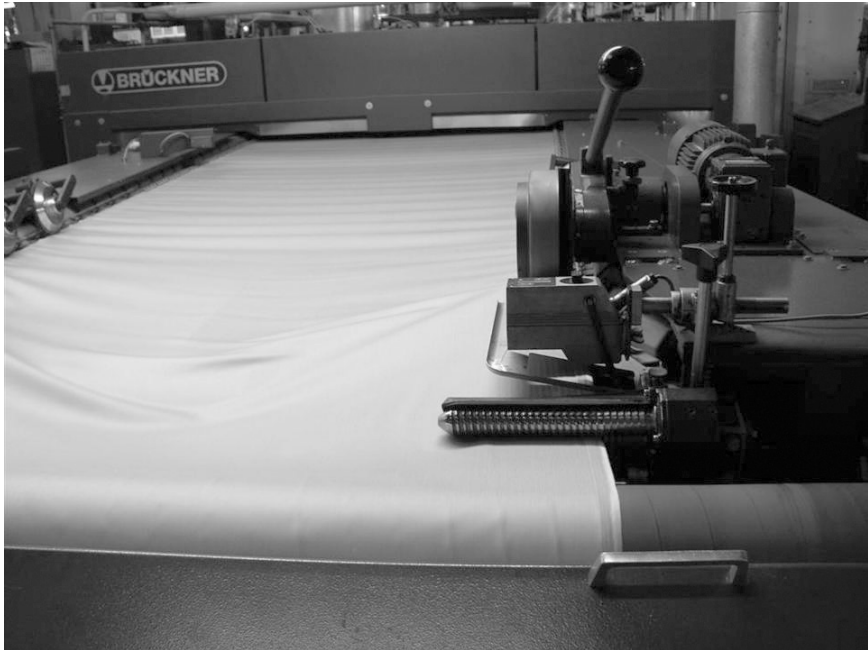
2.59 Shrinkage of fabric for dimensional stability.
