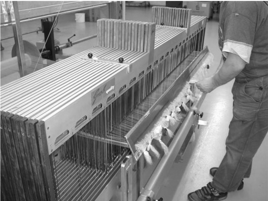
3.24 Warp yarn in weaving reeds, ready for knotting.
