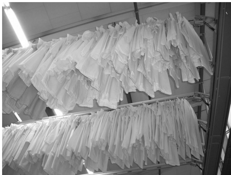
3.55 Cleaned laundry after tunnel finishing (drying process).
