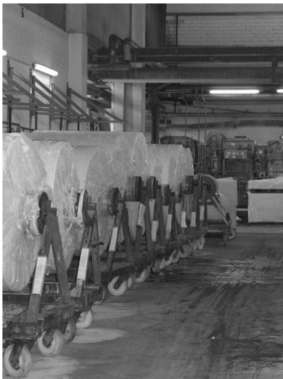
3.33 Pad cold patch treatment, an energy-efficient treatment for dyestuff development, simply by rotation overnight.
