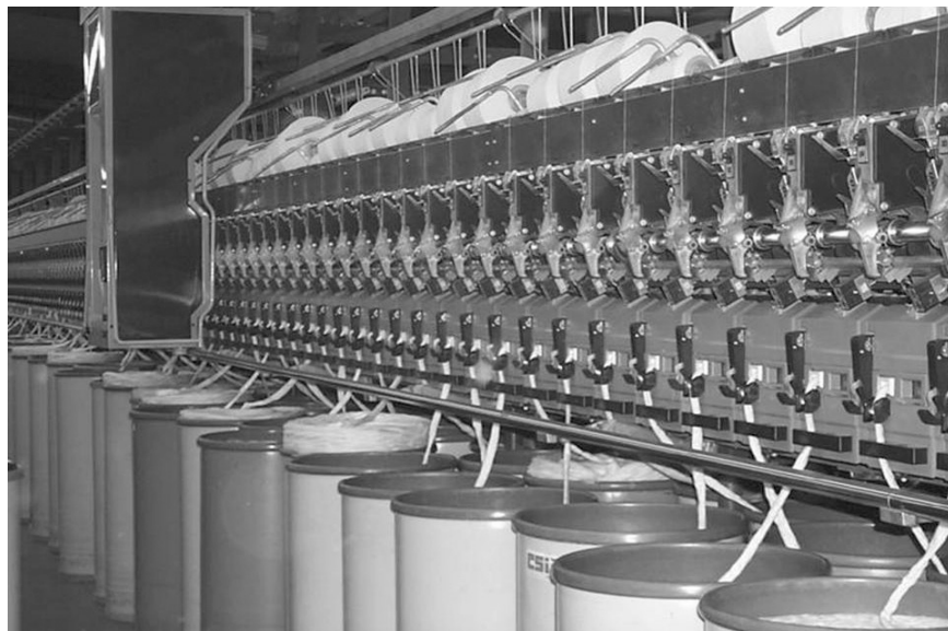
3.15 OE spinning from cans with carded sliver. A travelling piecing robot repairs ends down.
