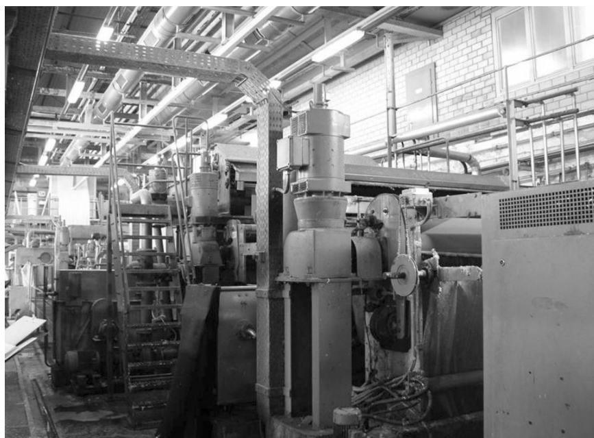
3.28 Pre-treatment machinery as applied for an elastic cotton 'Manchester' fabric (case study E in Chapter 4).
