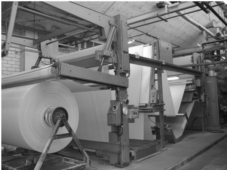
3.30 Open processing of a cold padded fabric. After the fixation of the applied dyestuff on the rotating roll (in front), the fabric is conveyed to a washing and rinsing process for removal of excess dyestuff.
