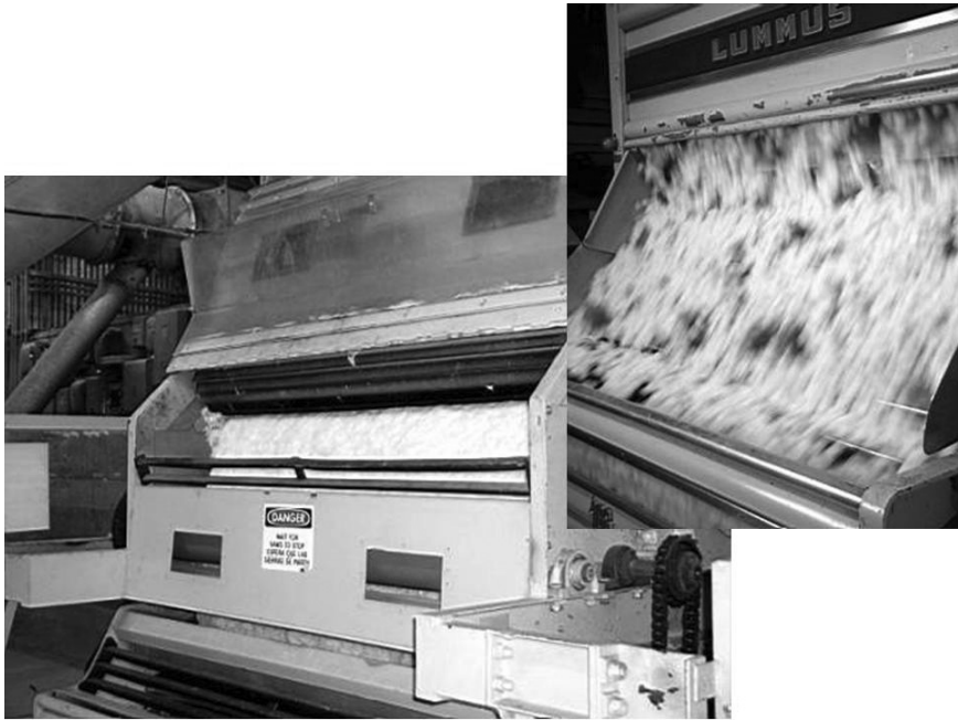
2.28 Saw gin for separating fibers and seeds. The insert shows cotton flocks in movement (source: Simone Schaerer).
