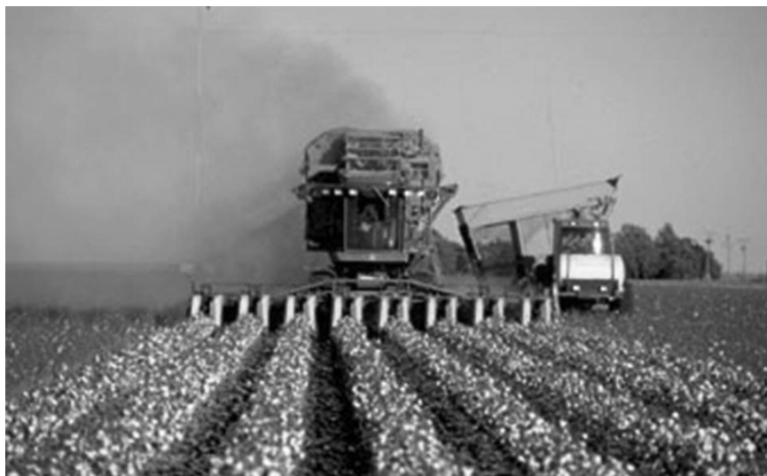
2.9 Harvesting machinery for stripper cotton in the Texas High Plains.
