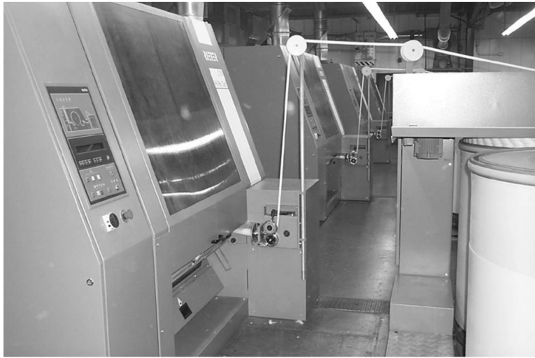
2.43 The carding process in cotton spinning for sliver production. The sliver has a fineness of 5000–6000 tex.
