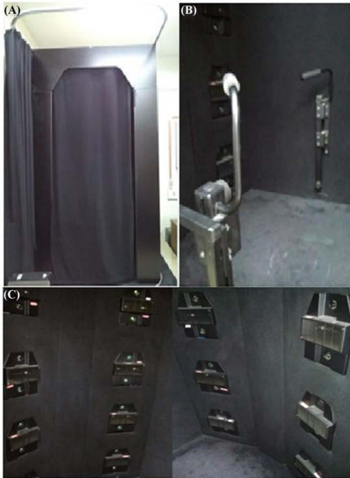
Figure 8.1 Images of the 3D body scanner. Panel (A): Outside view; Panel (B): Inside view, and (C) camera implanted inside the scanner to capture the 3D images.
