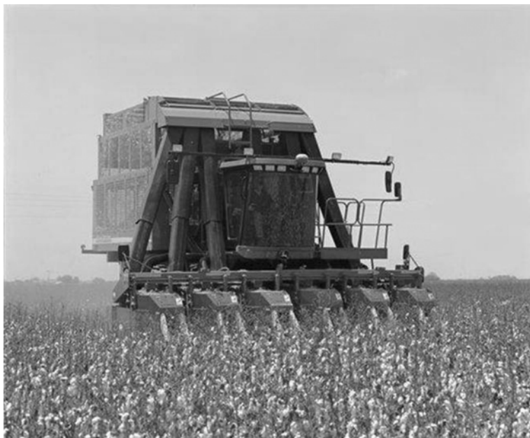
6.3 Typical spindle-type mechanical harvester for cotton.
