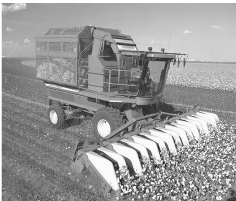
6.4 Typical stripper harvester for cotton.
