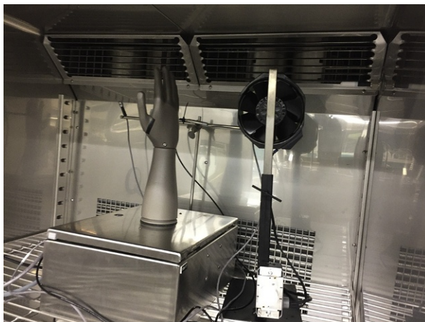
Fig. 4.7 Thermal sweating hand test setup at the CTT Group.
