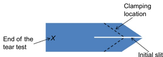
Fig. 2.30 Wing-shaped test specimen.
