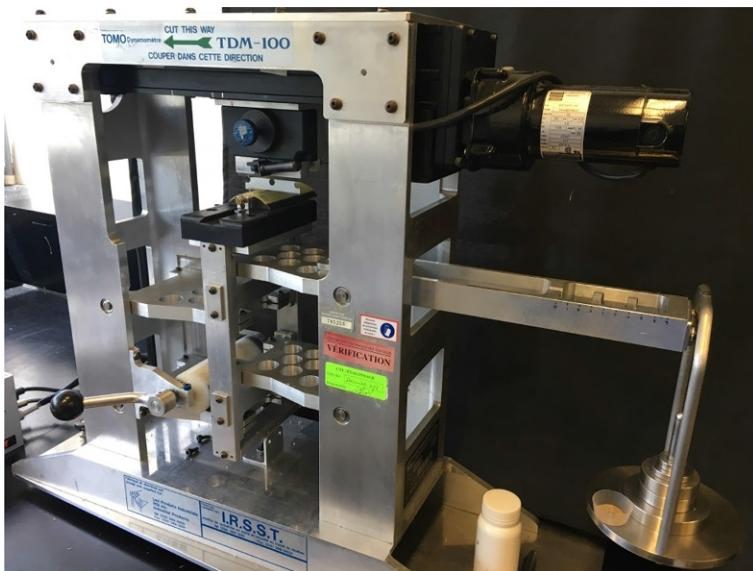
Fig. 2.34 TDM proposed for cutting resistance measurement. Courtesy CTT Group, QC, Canada.
