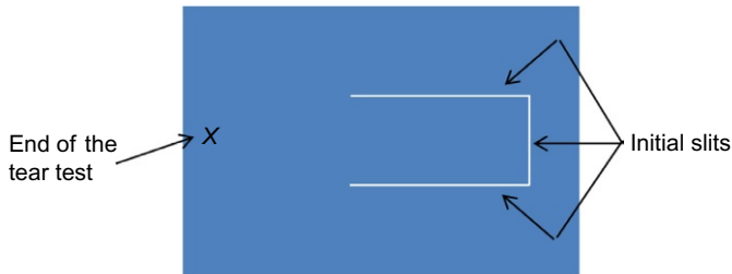
Fig. 2.32 Shape of the double tear tongue-shaped test specimen. Based on NF EN ISO 13937-4: 2000. Textiles—Tear properties of fabrics—Part 4: Determination of tear force of tongue-shaped test specimens (Double tear test).
