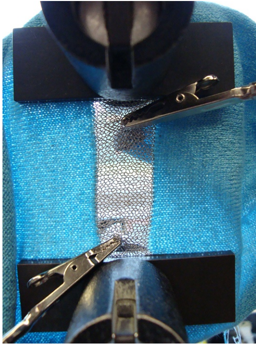
Fig. 12.5 Measurement of the electrical resistance of a conductive fabric under tensile stress.
