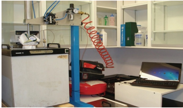
Fig. 9.6 Hot water immersion with a compression testing device (Mandal et al., 2014).
