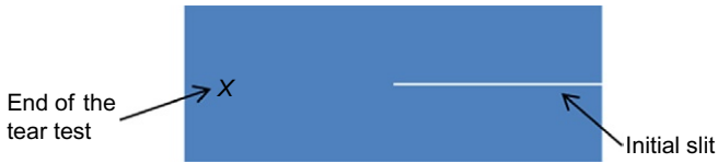
Fig. 2.27 Trouser-shaped test specimen.
