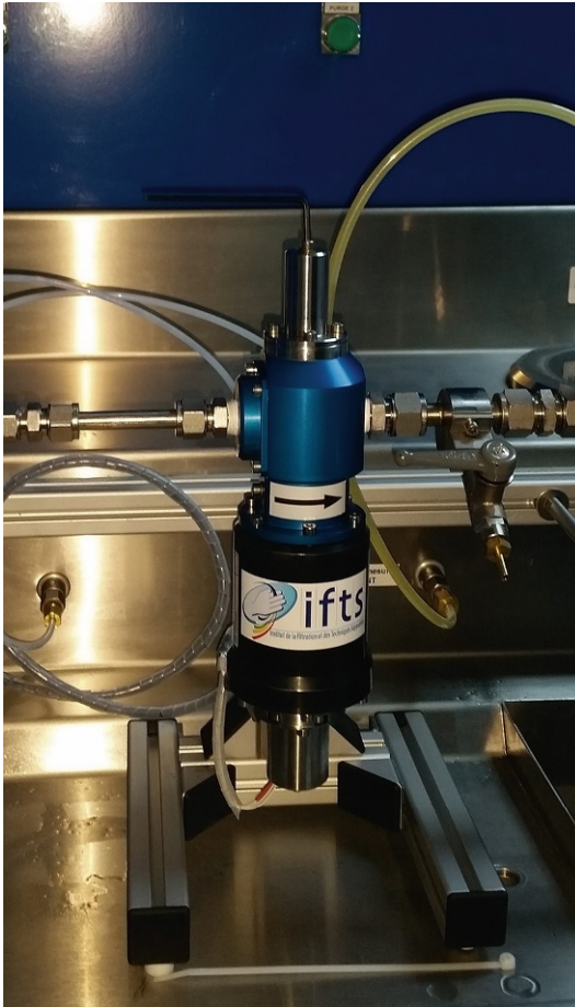
Fig. 13.19 Existing equipment generating automatic calibrated orifice as per ISO/TS 16332 (2017) . EDGE prototype—courtesy from IFTS.
