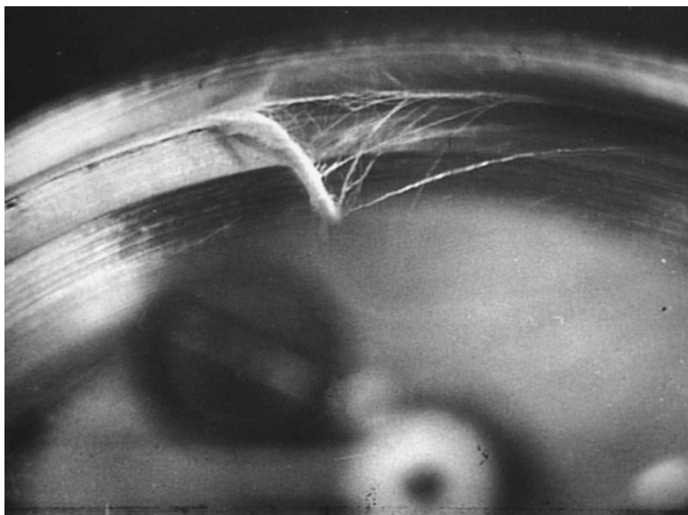
FIGURE 6.45 Wrapper fiber formation.
