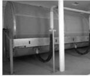
Rotary filter filters the air and separates fibres
