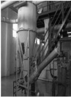
Centralized waste unit collect wastes from different machines in blow room
